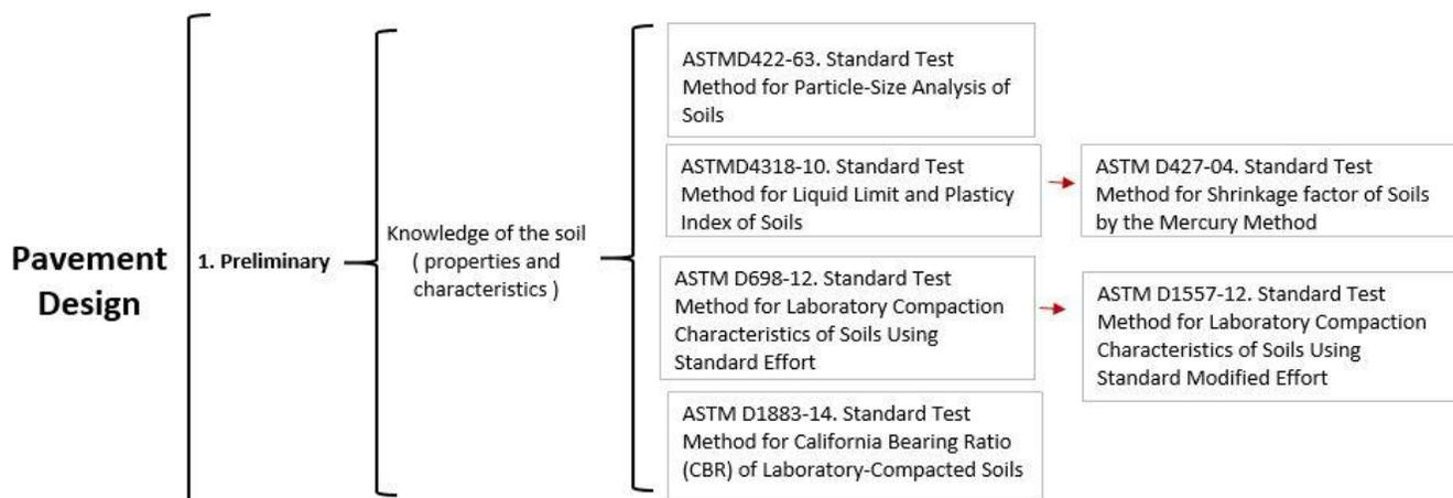
Fig. 1 Portion of the Process of Pavement Design (Preliminary Phase)
