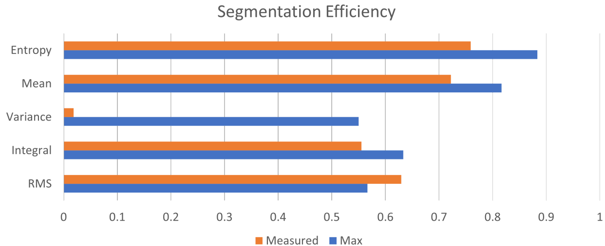
Fig. 3. Efficiency comparison of sEMG signal segmentation methods. The bar graph illustrates the segmentation efficiency for various computational methods, including Entropy, Mean, Variance, Integral, and RMS, comparing measured efficiency values against their respective maximum potentials. Entropy demonstrated the highest efficiency (0.88), confirming its robustness across different exercise sets, while Variance had the lowest performance, indicating inconsistencies in diverse exercise scenarios. The findings support the effectiveness of non-linear methods, particularly Entropy, in enhancing EMG signal segmentation accuracy.
