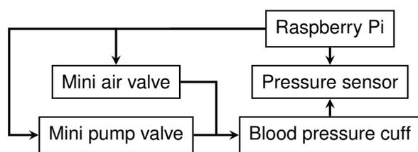
**Fig. 1.** BP module used for data acquisition
