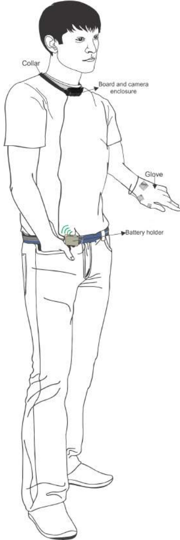
Fig. 15. Complete system. The image shows a user wearing the full system. The board enclosure and camera hanging on the neck, the battery holder attached to the belt and the gloves
