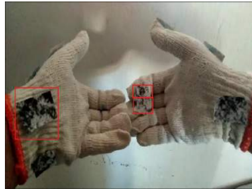
Fig. 8. Mexican sign language of the word “calle” and its adaptation in the gloves to characterize it. The red boxes show the chosen areas to place the patterns to characterize this sign
