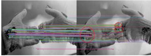
Fig. 9. Feature detection and matching between the fixed pattern for the sign “calle” (left) and the same sign performed afterwards
