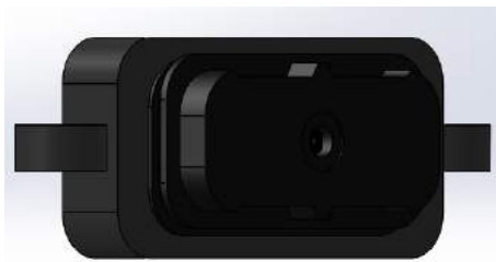
Fig. 13. Design of the board and camera enclosure. This enclosure is held by a pendant along the neck
