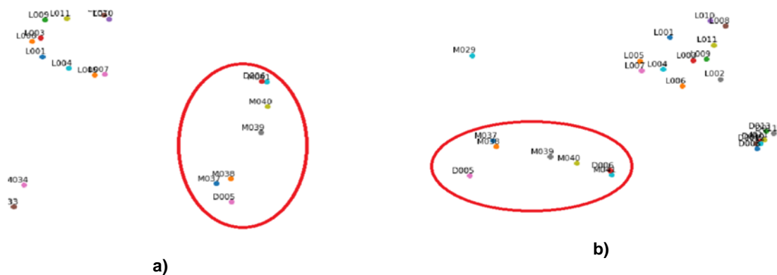
Fig. 5. Extract from the t-SNE plot for Kyoto-11 Dataset of CASAS, with (a) 60 seconds and (b) 600 seconds as the interval. In both cases we can see the sensors D005, D006, M037 to M040, which are in the toilet area, having similar activity
