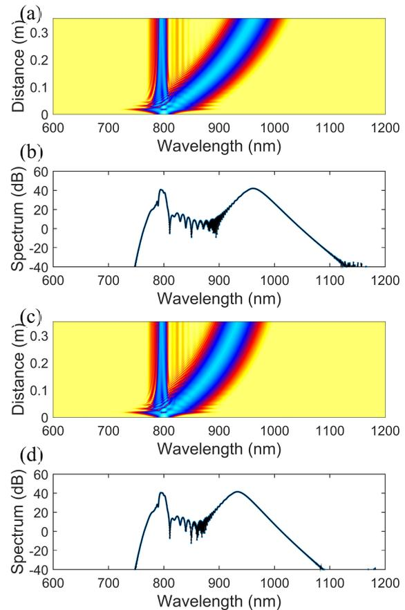
**Fig. 2.** (a) and (b) SC generation evolution and output spectra using the conventional model. (c) and (d) SC generation evolution and output spectra using our new pulse propagation model for  $L = 35 \text{ cm}$
