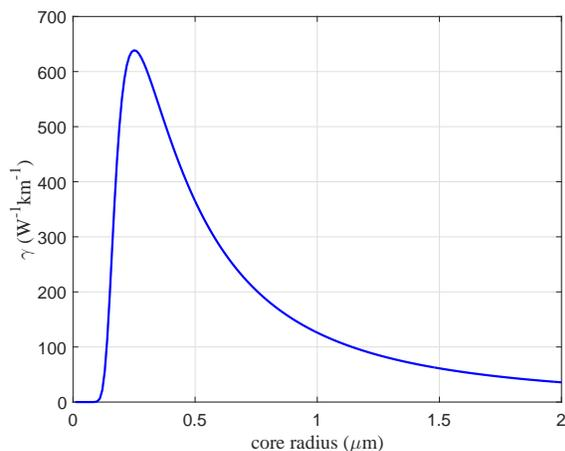
**Fig. 1.** Nonlinear parameter changes abruptly with the core radius of the air-silica photonic nanowire
