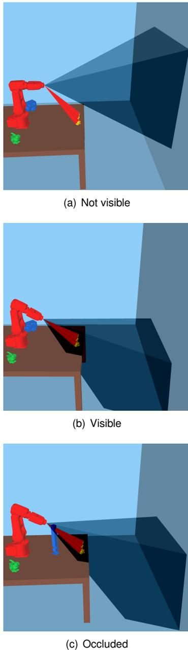
**Fig. 2.** Frustum model: camera frustum attached to the robot end effector. Ray-casting model: rays from the camera center to an object. (a) Landmark not visible by the camera: the Ray-casting model is not within the frustum model, (b) landmark visible by the camera: the Ray-casting model is within the frustum model, and (c) landmark occluded inside the camera field of view: the Ray-casting model collides with an object model
