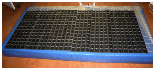
Fig. 2. Pressure sensor array of 32 \times 16 units in an area of 1108 \times 554 mm
