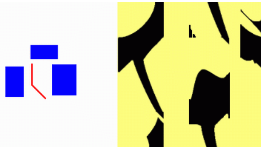
Fig. 2. A planar two-revolute joint manipulator arm
